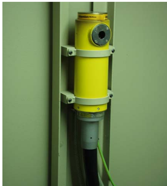
Figure 5. Photograph of a conventional x-ray tube used in a RTR system.
