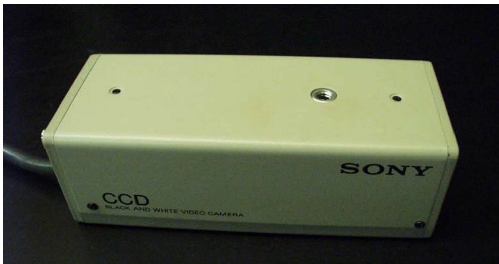
Figure 11. Picture showing one of the many commercially available CCD cameras that can be used for RTR. A lens would be attached to the right side of the camera and focused on the image intensifier output screen. The signal from the camera is then fed to a monitor for viewing.
